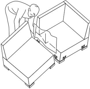
Line up the corner element with one of the adjoining units. Always lay a piece of our transport foil between the elements! This serves to smooth the alignment process and also prevents the upholstered covers from rubbing against each other and forming wrinkles. It is important to lift the elements slightly at the back, in view of the furniture's centre of gravity.
