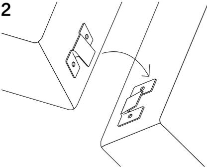
Raise the two units simultaneously and lower them again simultaneously! The fittings now engage with one another to hold the elements together (it is easy to disconnect them by lifting them up again).
